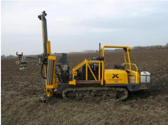
Figure 3.2: A cone penetration test
