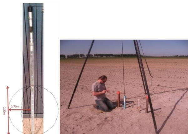
Figure 3.4: EM-Slimflex tool (left) and measurement (right)
