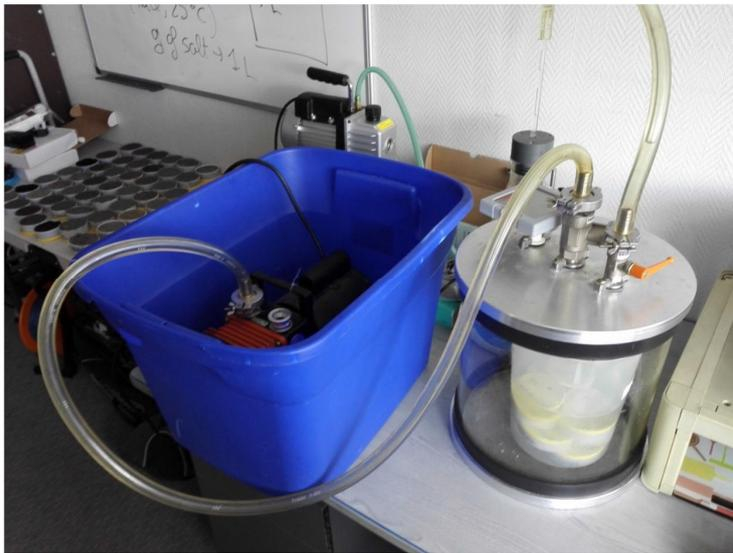
Figure 8.4 Saturation of samples under vacuum
